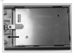
Figure 2-8 Remove HDD module
